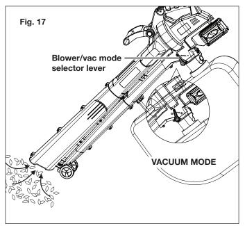
With a firm hold on the vac, tilt the tube 5 – 10 cm from the ground and use a sweeping action to collect light debris. The debris will flow into the bag. Items such as small leaves and twigs will be mulched as they pass through the fan housing. For longer bag life and increased performance, empty the bag frequently.
