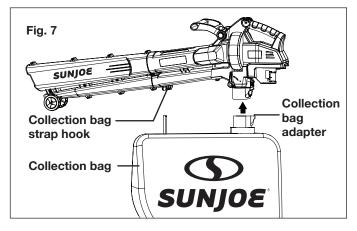
To remove the bag, simply press the bag releasing button, and pull the bag off (Fig. 8). Detach the strap from the strap hook.
