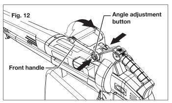
2. Release the angle adjustment buttons and the front handle will reset to lock into position automatically.
