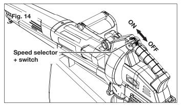
**3.** To stop the tool, slide the speed selector + switch backward until the notches in the housing align with the 0 position (Fig. 15).
