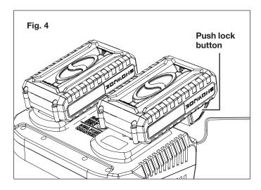
**CAUTION!** FIRE HAZARD. When remove the batteries from the charger, be sure to unplug the charger from the outlet first, then remove the batteries from the charger.
