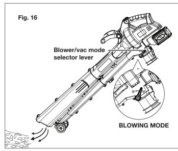
Hold the blower firmly with one hand on the rear handle and the other hand on the front handle. Sweep from side to side with the wheels on ground.  Slowly advance the unit by the wheels, keeping the accumulated pile of debris in front of you. Most dry blowing operations are better suited to low speeds rather than high speeds. High speed blowing is best for moving heavier items like large debris or gravel.
